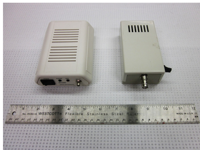
Fig. 2. Avicenna RX1200 Digital Multichannel Analyzer (left) and high voltage power supply (right).
