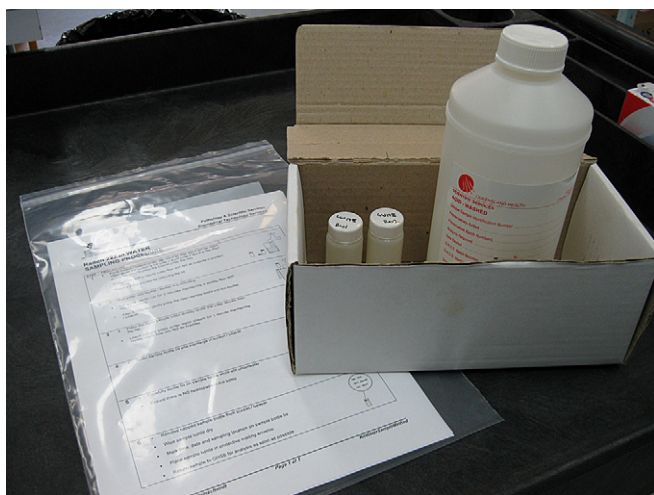
Fig. 1. Groundwater sampling kit including 1 × 500 mL acid washed polyethylene bottle, 2 × 20 mL Teflon coated polyethylene liquid scintillation vials, sampling instructions and questionnaire, and reusable shipping container with prepaid consignment note.
