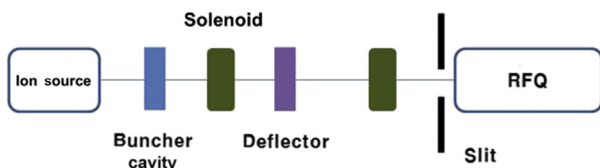
Fig. 1 – Schematic layout of a pulse proton beam generation system. A deflector is located between two solenoids and a slit is located in front of the radiofrequency quadrupole (RFQ). A buncher cavity is placed after the ion source and the distance between the buncher and the slit is determined to maximize modulation of the beam current at the slit position.
