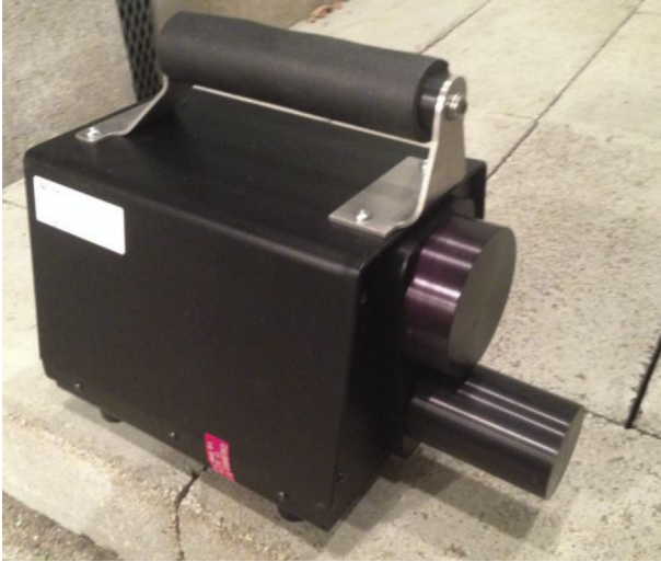
Fig. 1. N-Probe fast and thermal neutron spectrometer (Ing et al, 2007).
