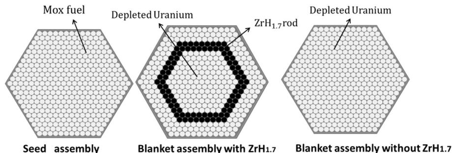
Fig. 1. Types of fuel assembly loaded in the core of super FR.
