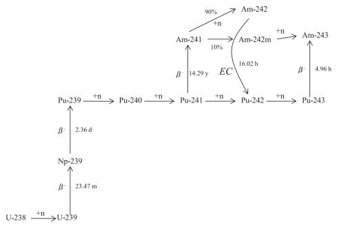
Fig. 1. Production of americium isotopes in a nuclear reactor. Only reactions and decays that lead to americium are shown.
