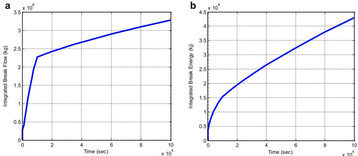
**Fig. 1.** (a) Distribution of integrated mass flow (water and steam) Released with time, (b) Distribution of integrated energy released with time (The AP1000 European DCD, 2007a).
