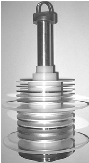
Fig. 1. The TRR corrosion test rack.
