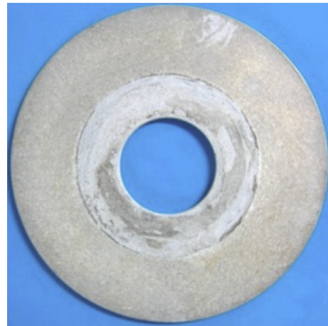
Fig. 3. Outer surface of single 6061 Al alloy coupon after 6 months of exposure in the TRR reactor.
