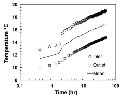
Fig. 2. Circulating fluid temperatures during an in situ thermal response test.
