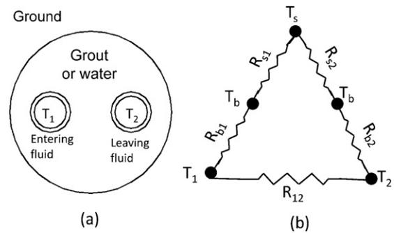
Fig. 1. (a) Borehole geometry and (b) thermal resistance model.
