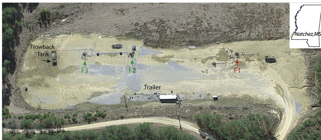
Fig. 1. Aerial view of the detailed area of study at Cranfield site (Lon: -91.141^\circ , Lat: 31.564^\circ ), which consists of an injector (F1) and two monitoring wells (F2 and F3). During leak experiments, F3 was used as a “leaky” well. Locations of the flowback tank and trailer area are also labeled.
