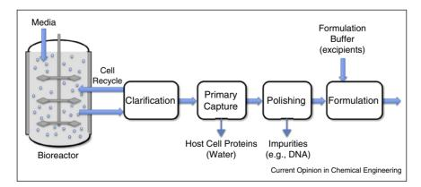
Schematic representation of a generic continuous downstream bioprocess. Source: Adapted from Ref. [16\*\*].
