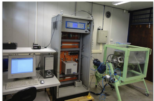
Fig. 1. Structure of the composting experiments that, basically, comprise a rotary reactor, a gas analyzer and a microcomputer to retrieve data.
