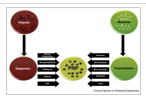
Schematic overview of polymer nanoparticles synthesis methods by either polymerization from monomers or preparation from preformed polymers. SCF: supercritical fluid technology, C/LR: controlled/living radical. Image taken from Rao and Geckeler [10\*\*].
