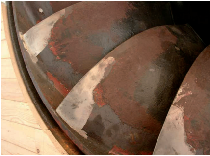
Figure 2. Completed replacement of leading edges damaged by cavitation following extensive repair work.
