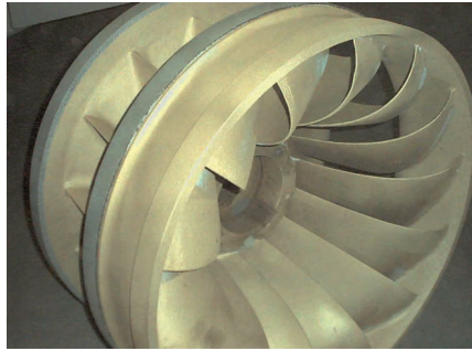
Figure 3. Francis turbine following preparation by grit blasting.
