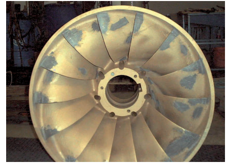
Figure 4. Turbine following rebuild using a paste-grade material to in-fill areas of erosion damage.
