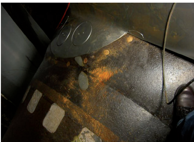
Figure 1. Damage to hub of a Kaplan turbine (L) and close up of the damage (R).
