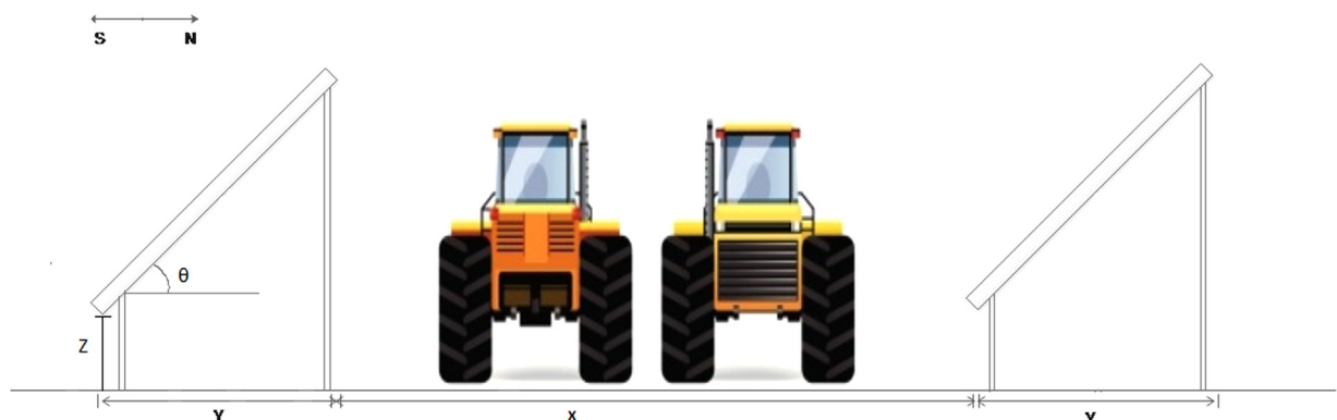
Fig. 1. Agrivoltaic farm schematic having ground mounted PV modules with the area between the panels being used for farming. The spacing between the PV modules has been kept wide enough to allow standard sized farming equipment to pass between the rows.
