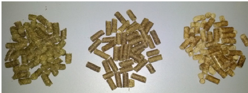
Fig. 1. Samples of olive waste pellets for different moisture contents 24.4%, 26.7% and 23.2% respectively [26].
