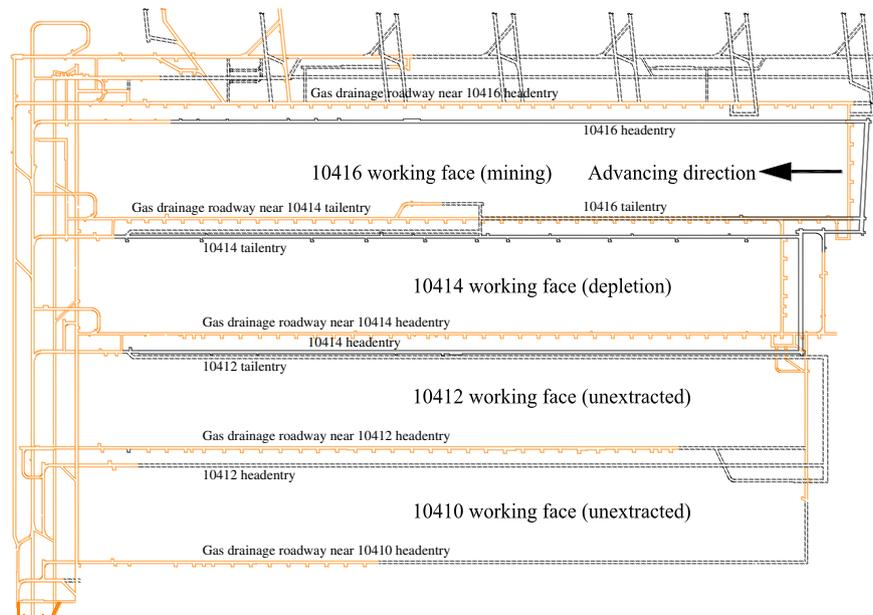
**Fig. 1.** Plan view of the 10416 working face of the 104 mining district (owing to size limitations, the four working faces below 10410 have been omitted (i.e., 1042, 1044, 1046, and 1048).
