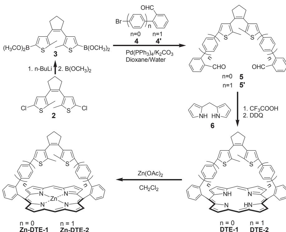
Scheme 1. The synthetic procedures for the hybrid DTE-1, DTE-2 and their zinc complexes.
