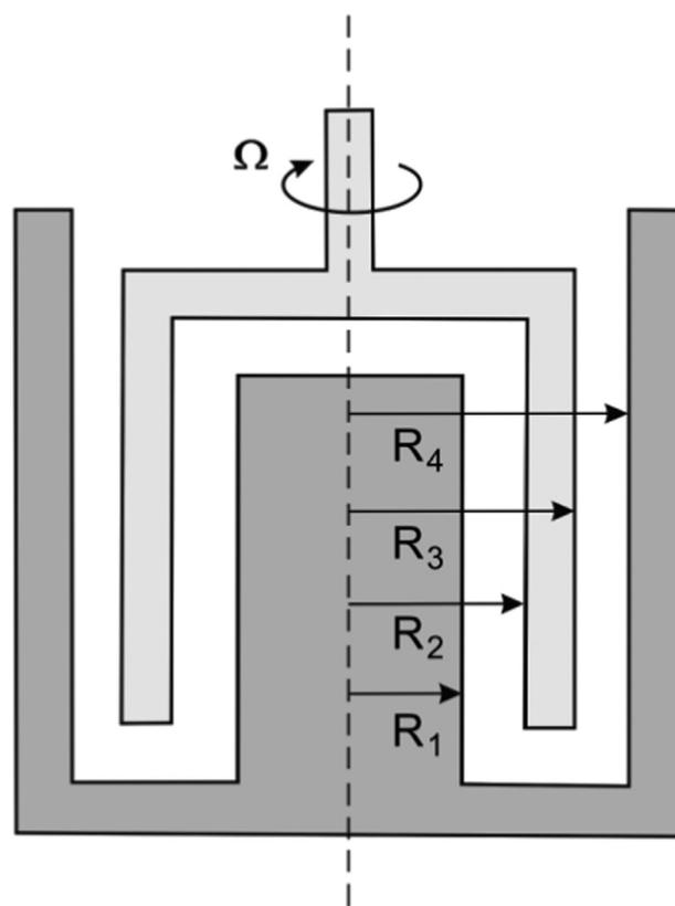
Fig. 2. Scheme of the double-gap cell used in the HDR experiments carried out in the rheometer, being:  $R_1=8.88$  mm,  $R_2=9.18$  mm,  $R_3=10.50$  mm and  $R_4=10.85$  mm. The length of the rotor is 55.00 mm.
