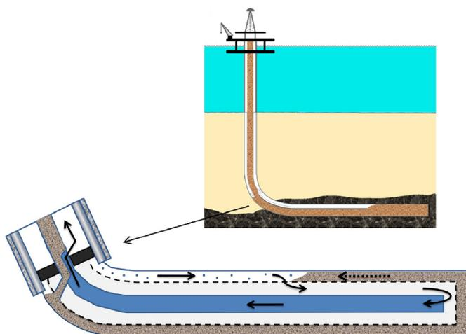
Fig. 1. Scheme of a gravel filling (adapted from Magalhães et al., 2006).
