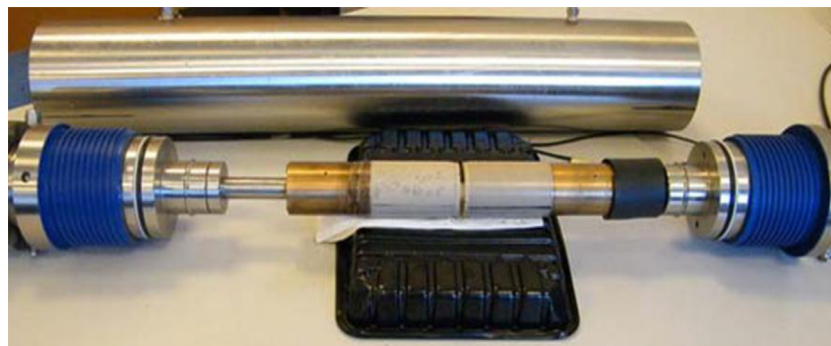
Fig.1. (A) Steel cylinder casts designed for high pressure use, (B) the mineral mix as a fine powder, (C) hydraulic compressor with different steel blocks and hydraulic pressure jack used to create synthetic shale, and (D) Synthetic shale core samples with different percentages of TOC from 0% to 20%.
