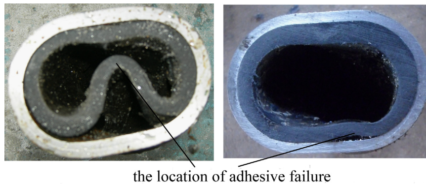
Fig. 1. Cases of adhesive failure of even thickness PCP used in Daqing oilfield.
