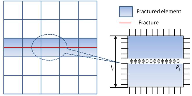
Fig. 1. Demonstration of fracture elements in the geometrical model (left) as well as the load condition in one fracture element at the frozen time point (right).
