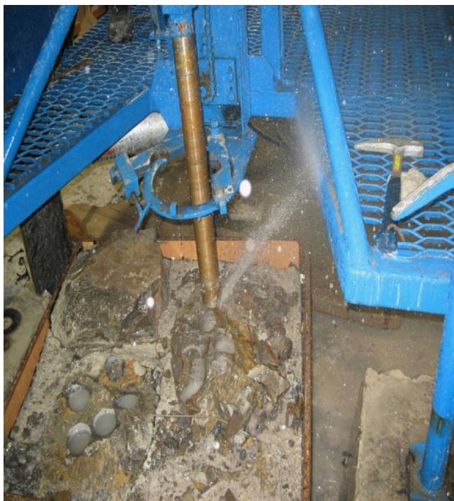
Fig. 2. Photo of laboratory setup for the drilling experiments.
