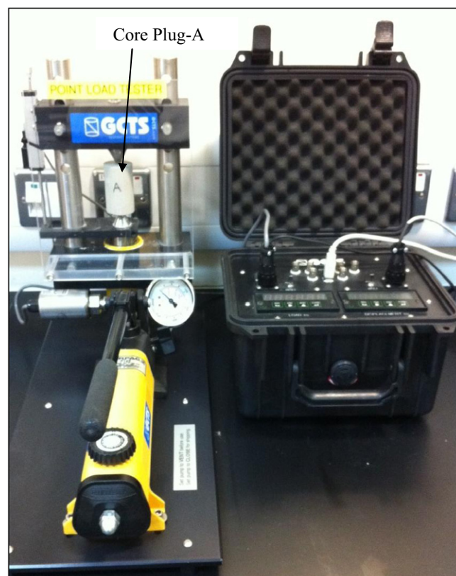
Fig. 1. Point load tester used for fracturing core plugs. Core plug top face of the fractured core plugs-A, B and C.
