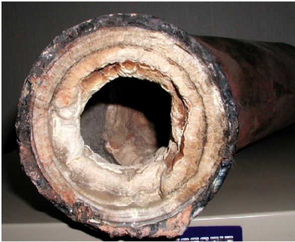
Fig. 1. The build-up of scale inside a tube.
