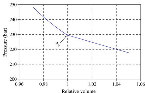
**Fig. 1.** Pressure–volume plot of mixture at 85 °C to determine its bubble point pressure.
