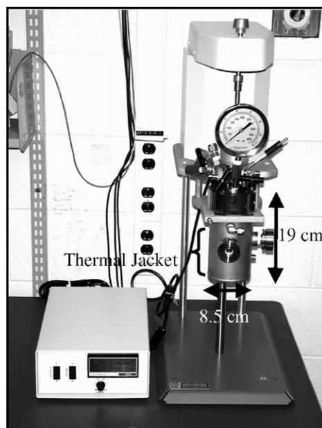
Fig. 1. The 450 mL Parr vessel with maximum working pressure of 21 MPa with two quartz windows. Shown to the left of the Parr vessel is the power supply for the magnetically driven impeller. Chilled ethylene glycol was used for temperature control and was circulated through a thermal jacket that surrounds the vessel.
