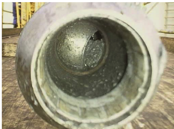
Fig. 1. The stuck ball valve of PTCS (Aumann and Associates, 2003).
