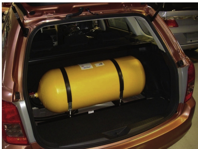
Fig. 1. A 30-L CNG cylinder mounted at the boot of a car.
