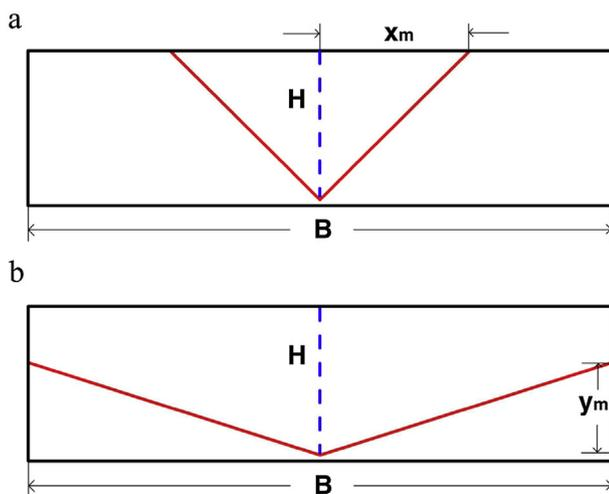
Fig. 1. Illustration of a triangle-shaped steam chamber: (a) steam chamber horizontal expansion and (b) steam chamber going downwards.
