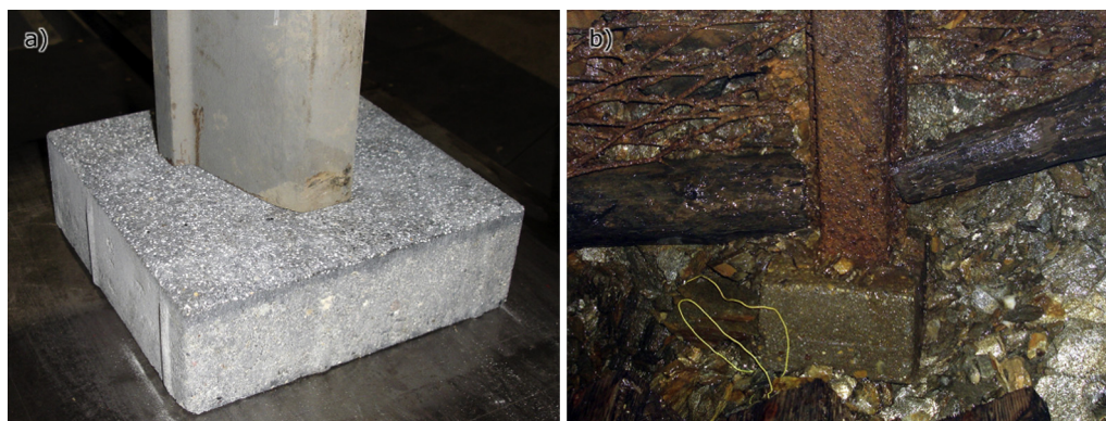
Fig. 1 – Bearing plates made of concrete a) concrete bearing plate prepared for stand test, b) concrete bearing plate in an old mine working.
