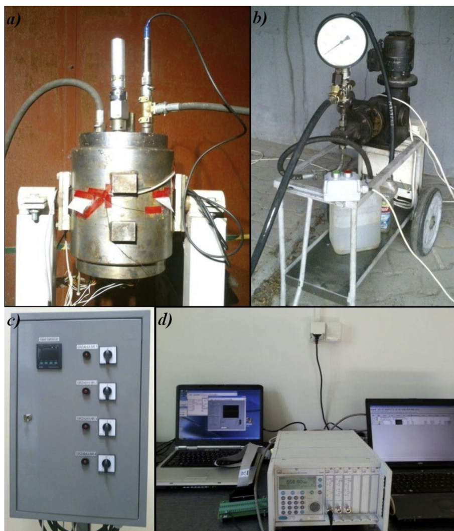
Fig. 1 – The stand for testing explosives: a) chamber for tests of explosives. b) switch board of power breaker. c) hydraulic pump. d) set recording test results.
