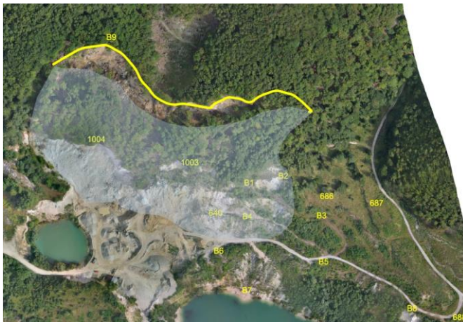
Fig. 2. Top view of the rock slide, its head scarp and arrangement of the observed points. The most active part of the rock slide is highlighted in white shading
