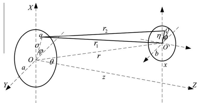
Fig. 1. Off-axis measurement geometry considered with transmitter of radius  $a$  and hydrophone of radius  $b$ . The transmitter surface is in the  $XY$  plane, and  $Q$  is a point on the hydrophone surface.
