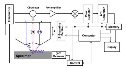
Fig. 1. Schematic diagram of SAM.
