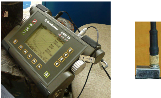
Fig. 1. UT instruments: Krautkramer's USM25 pulser/receiver device (on the left); and SMWB70-6 probe (on the right).
