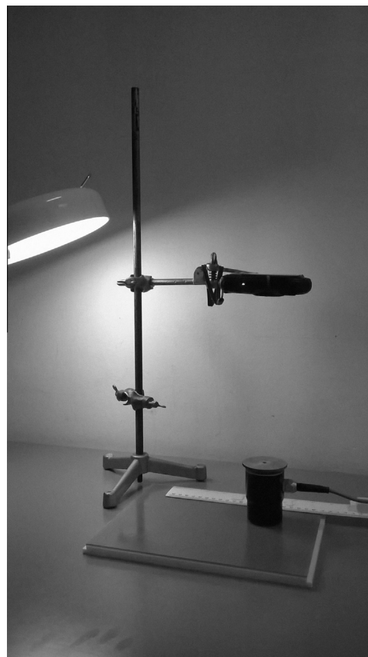
Fig. 1. Experimental set-up showing the thermochromic tile, transducer, weight, ruler and digital camera on stand.
