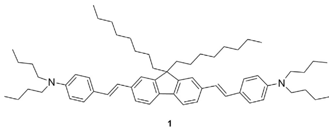
Fig. 1. Structure of a D– \pi –D chromophore based on a 9,9-bis(octyl)-fluorene core with reported TPA of 1140 GM [14].
