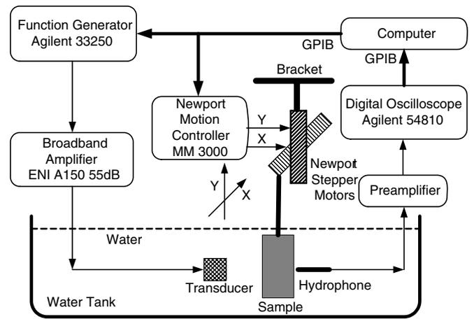
Fig. 1. Schematic block diagram of the experimental system.
