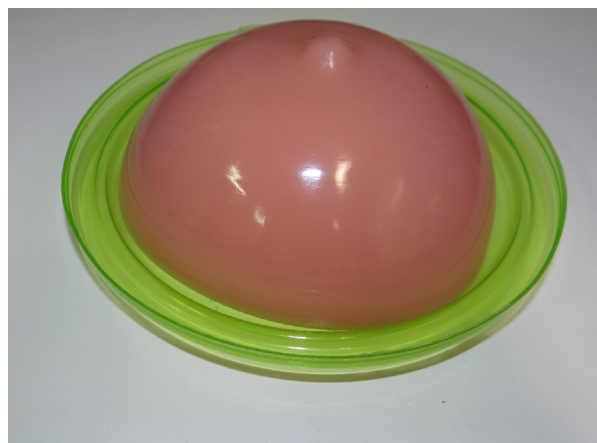
Fig. 1. Photograph of the paraffin-gel breast phantom.
