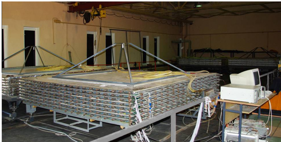
Fig. 1. The muon hodoscope URAGAN. In the foreground, one of the supermodules is seen. On the left and in the background the other three SM are located.
