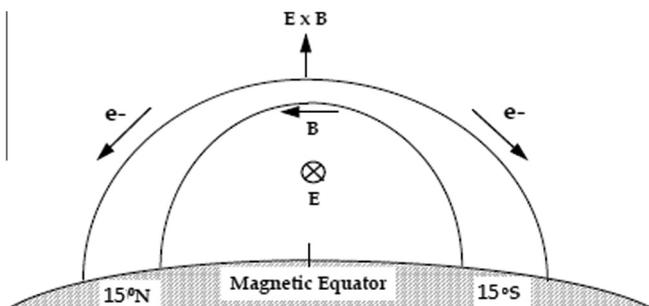
Fig. 1. Illustration of the equatorial fountain effect which gives rise to the equatorial anomaly. E and B represent the electric and magnetic field vectors respectively.
