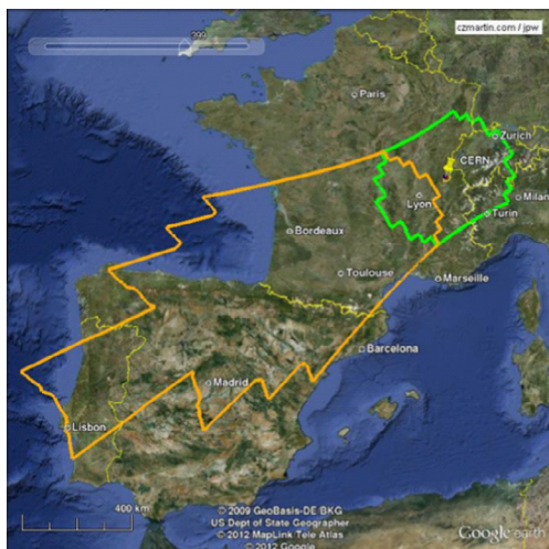
Fig. 2. Left: Footprint of the field of view of the JEM-EUSO telescope, projected to west Europe: Nadir mode (Green) and Tilted mode (Orange); Right: Expected time evolution of the exposure. Space-based missions JEM-EUSO can achieve the critical threshold of 10^6 \text{ km}^2 \text{ sr yr} . (For interpretation of the references to color in this figure legend, the reader is referred to the web version of this article.)
