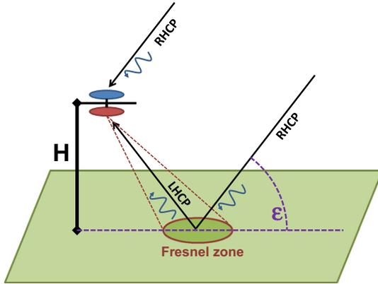
Fig. 1. Basic principle of GNSS-R. RHCP signals transmitted from a GNSS satellite are reflected on the Earth’s surface and change polarization (to LHCP). These signals can be received, analyzed and used to deduce geophysical parameters of the reflecting surface.
