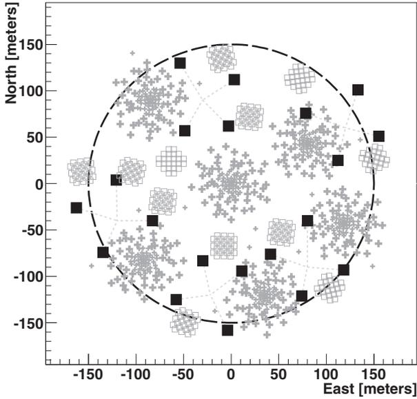
**Fig. 1.** Layout of the LORA array in the LOFAR core. The filled black squares represent the LORA detectors, the crosses the LOFAR low-band antennas and the empty squares the high-band antennas. The dashed circle in the figure illustrates the fiducial area of a radius of 150 m, which is used in the analysis.
