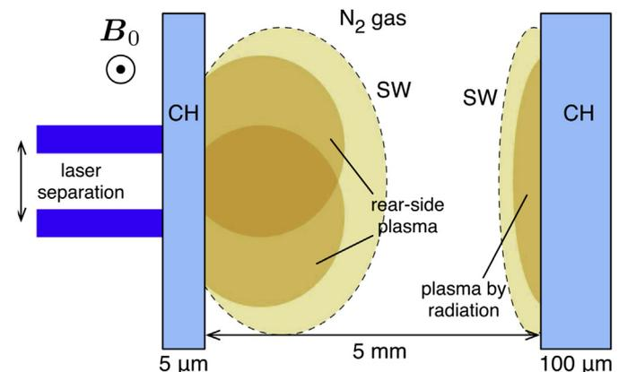
Fig. 1. Simulation condition of Richtmyer–Meshkov instability experiment in magnetized laser ablation plasma with double target configuration.
