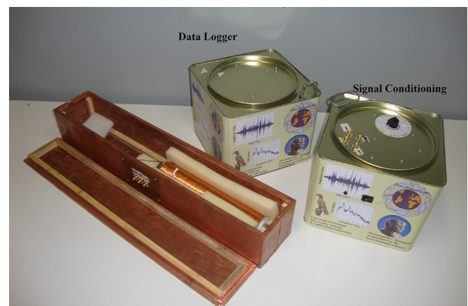
Fig. 1. Photograph of the proposed Schumann resonance detection system.
