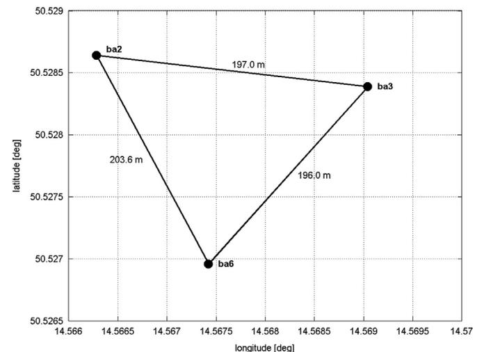
Fig. 1. Infrasound array at observatory Panska Ves. Position of sensors ba2, ba3, and ba6 is represented with circles. Distance between the sensors is shown.
