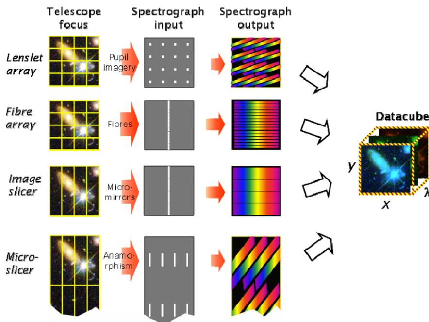
Fig. 1. A summary of the four main techniques of integral field spectroscopy.
