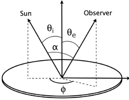
**Fig. 1.** The definition of the viewing geometry of a surface.  $\theta_i$  is the angle between the incident light and the surface normal,  $\theta_e$  between the observer's direction and the normal.
